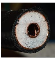
2. Using the Flat Bladed Screwdriver or the Utility Knife push the foam dielectric away from the center conductor. The test connector slips over the outside of the feedline center conductor and clearance must be made.
