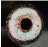
3. Strip 1.5" of the outer jacket off. The test connector slips over the outer conductor and not over the jacket.
